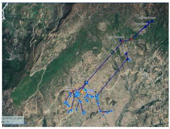
618,724.50. The scheme have 79 private taps, 4 public taps, 8 intakes, 5 reservoir tanks, 3505 m distribution pipeline and 4450 m transmission pipeline.
