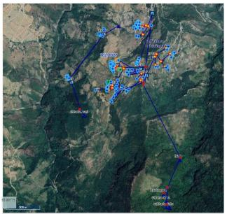
scheme has an additional cost for private tap connection as Users Cash: 800,000 Users in-Kind: 1,714,021. The scheme has 162 private taps, three public taps, six intakes, nine reservoir tanks, 5,630 m distribution pipeline and 5,574 m transmission pipeline.
